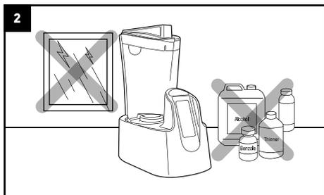
• The equipment should not be installed next to a heat source or in the face of direct hot air (tumble dryer, dishwasher, refrigerator, heater, boiler, etc.).
